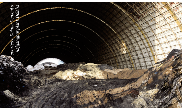
Fly ash needs activated lime available from cement clinker to become cementitious.
