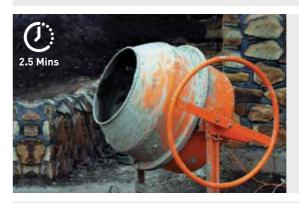
Good concrete is homogenous and is prepared by thorough mixing of all the ingredients. To ensure homogeneity in the concrete mix, it should be prepared in mechanical mixers and mixed for at least 2.5 minutes.
