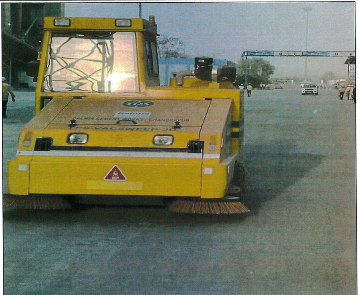
Mechanical Road Sweeper deployed for Road Cleaning
