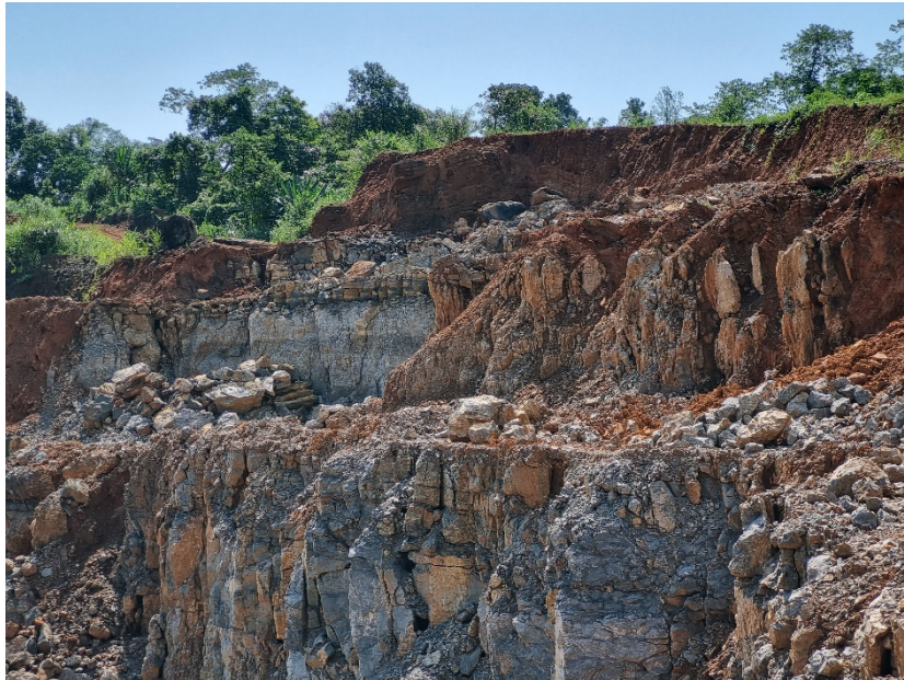
Fig. 19b. The exposure of the Umlatdoh Limestone and Nurpuh Sandstone at the top benches of the mine pit.
