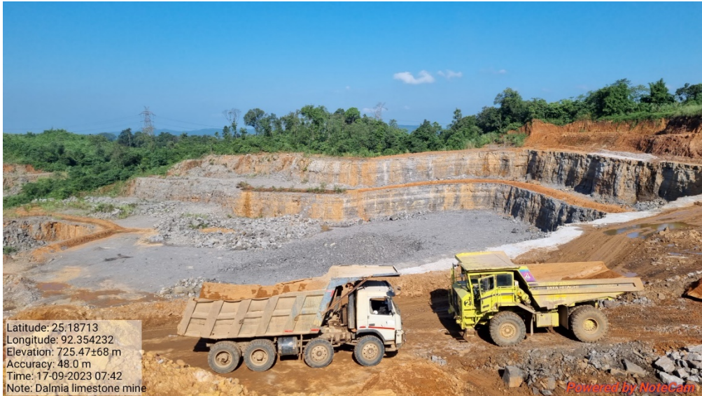
Fig. 18. Umlatdoh Limestone exposed in the mining benches.
