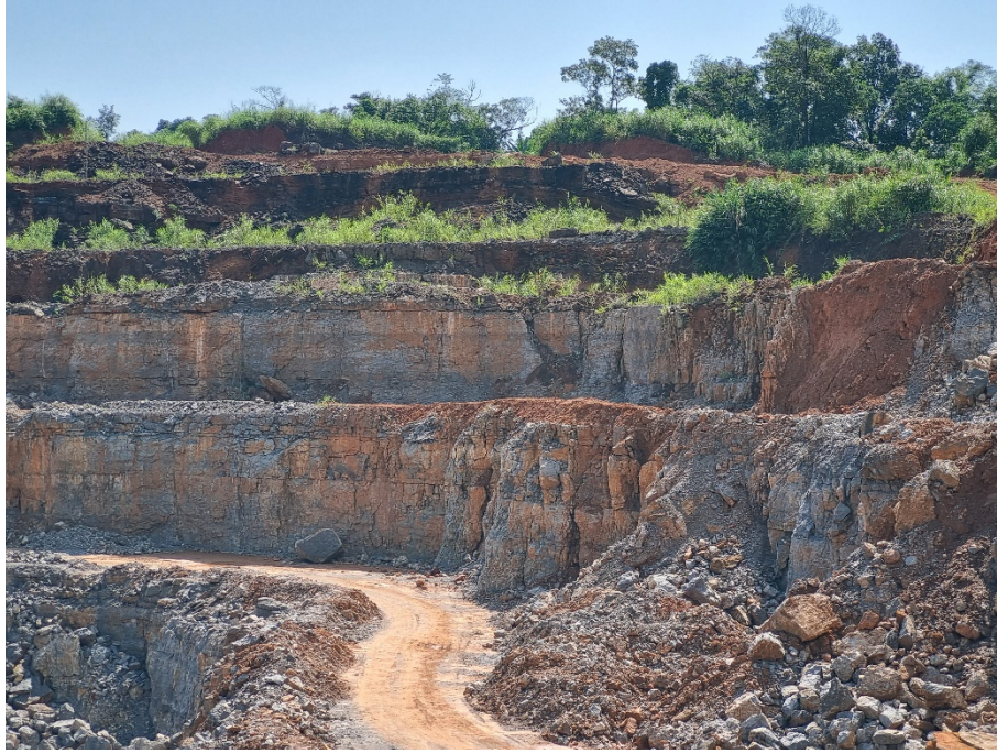
Fig. 17. Lakadong Limestone overlain by Lakadong Sandstone in the mine benches.
